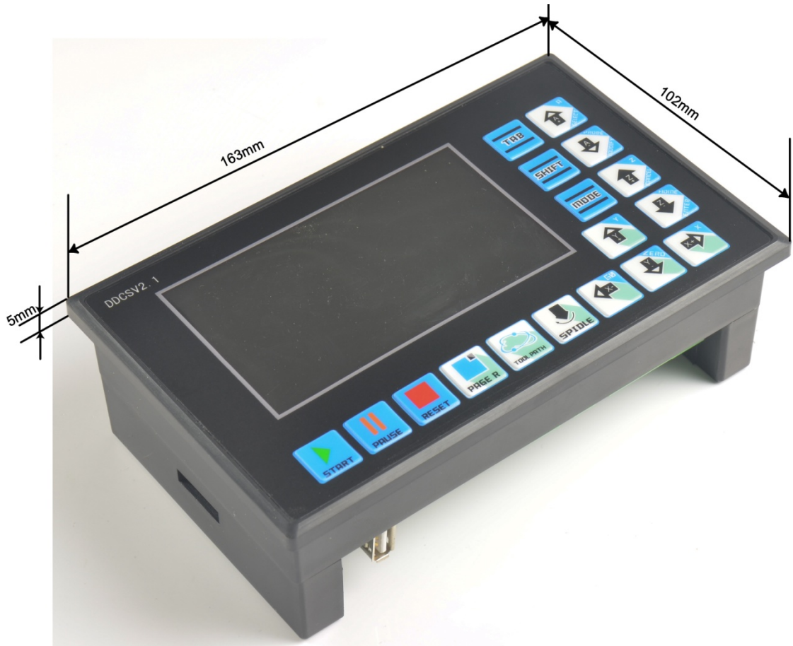
Picture1-1 DDCSV2.1Front external view and dimension figure
