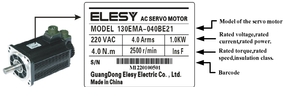
Figure 10-1 Servo motor nameplate description
