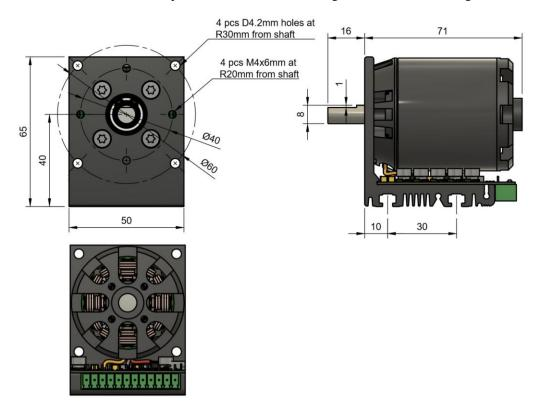
Positive rotational direction is clockwise rotation when looking at the motor front plate (as shown above in the top left picture).
