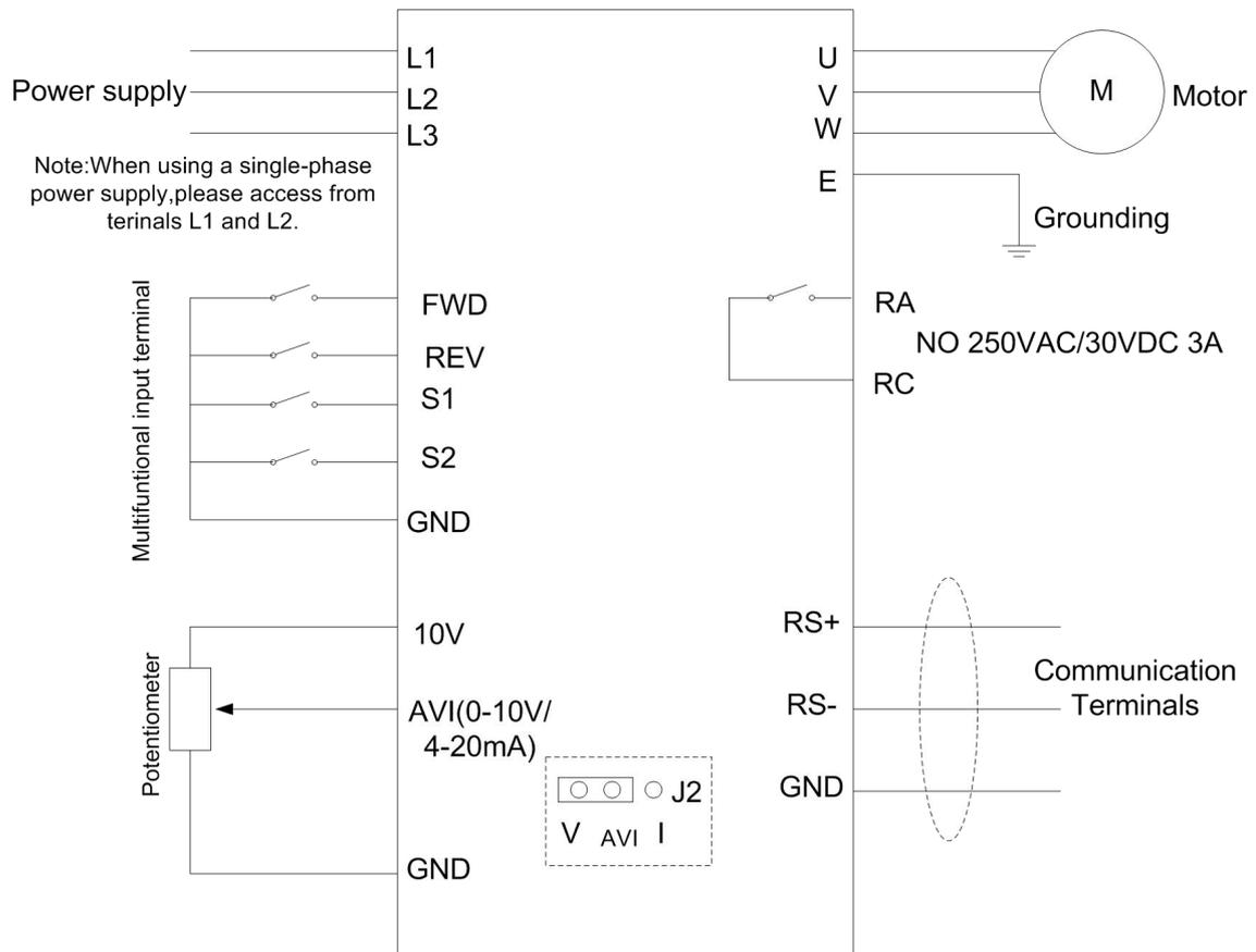
Note: AVI terminals can be used to select an analog voltage input (0-10V) and analog current input (4-20mA) through the switch J2.
